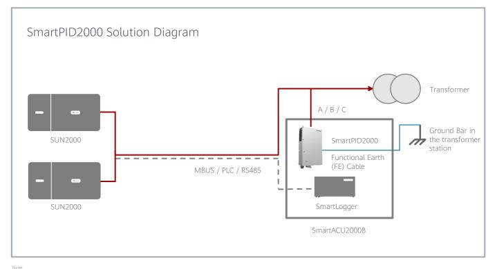
Note: 1. The Anti-PID solution could ONLY be deployed in utility installations which are normally connected to the medium voltage (MV) grid running WITHOUT neutral line. 2. The Anti-PID module must work with Huawei SmartLoggers and Huawei inverters.
